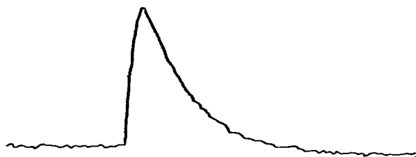
Fig. 1. Calorimetric heat burst curve for a 1 millicalorie exothermic reaction.
